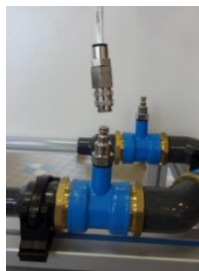
Illustration of a pressure tap by self-closing quick coupling
