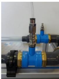
Illustration of a pressure tap by self-closing quick coupling
