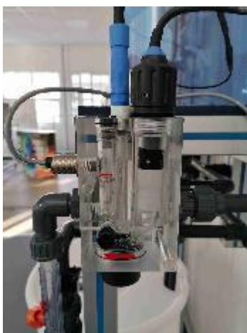
Option GPBT73 : Chlorine regulation system with Cl 2 probe and pH probe
