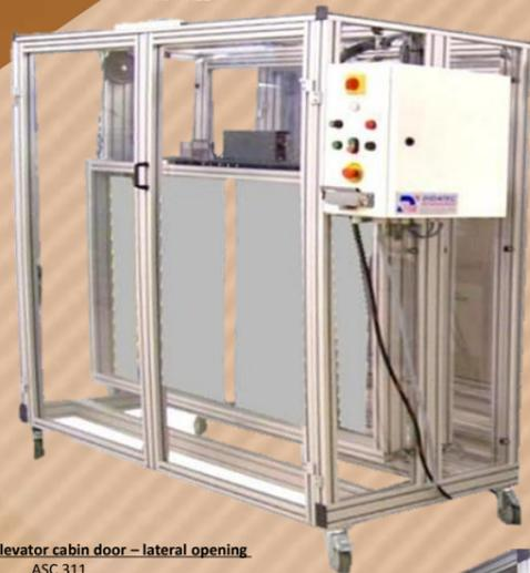
Landing door and elevator cabin door - lateral opening
