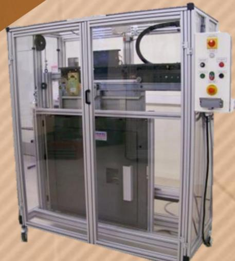
Swing landing door and elevator cabin door-lateral opening
