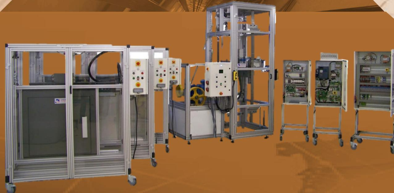
Inverter elevator maintenance with operative part
