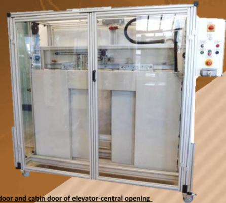
Landing door and cabin door of elevator-central opening
