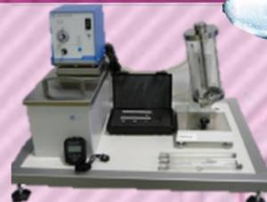
Falling ball viscometer
