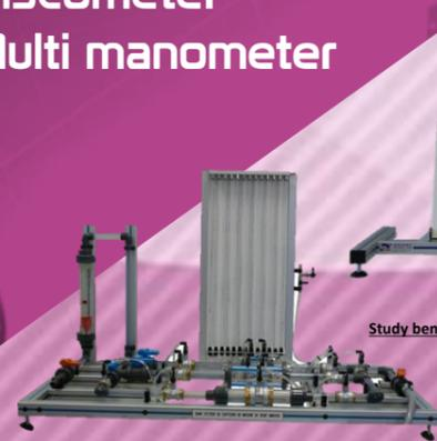
Study bench of flow rate measurement sensor
