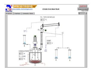
We find in this window the block diagram of the machine with the location of various measures of temperature and their values.
